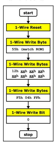
The following diagram shows how to turn off the switch.
