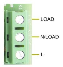
Connect the 230 V or 120 V mains between N/LOAD and L.
