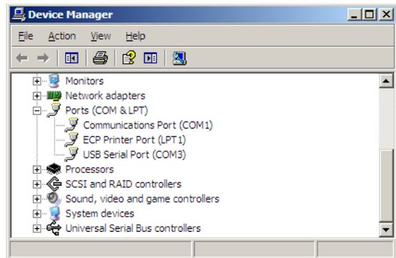
The device name of a serial port is shown between parentheses. In the picture to the right, you can see two serial ports. COM1 is the PC's on-board serial port, COM3 represents a USB serial adapter.
